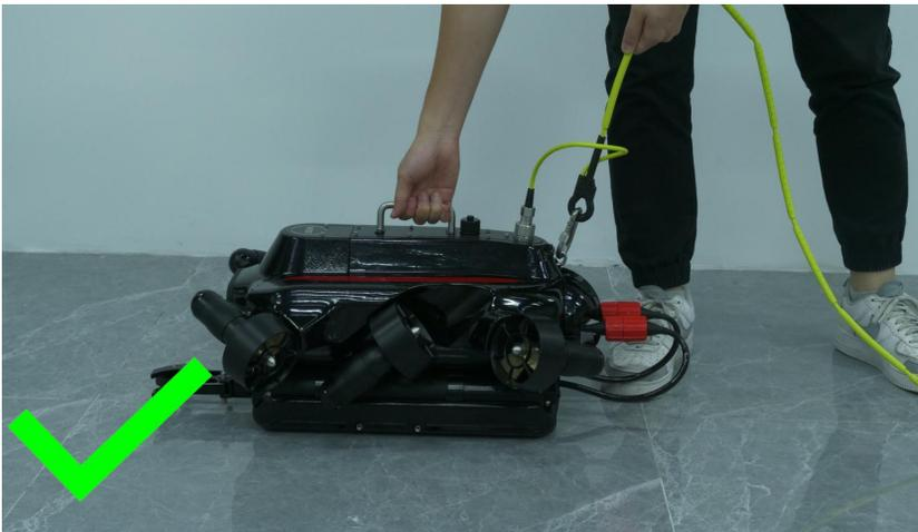
Holding the LAR handle and tether behind safety lock when launch or recovery
