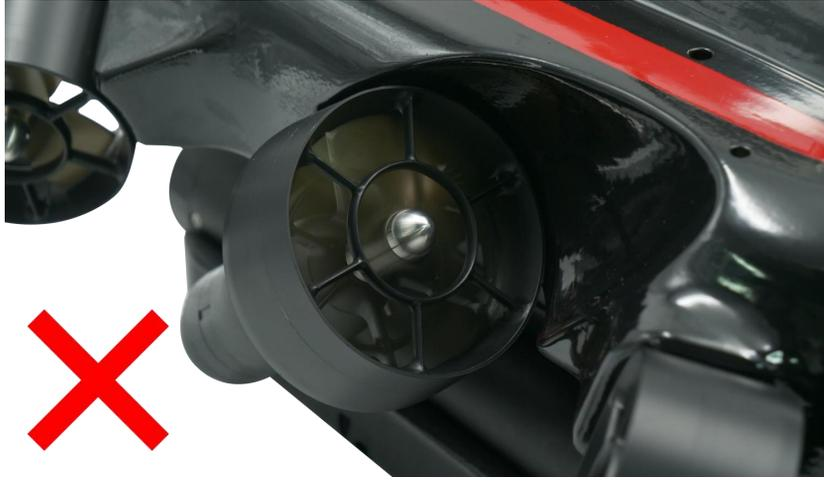
Do **NOT** unlock the motor in air over 3 seconds, to avoid over heating
