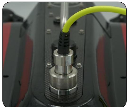
3.2.3.2 insert ROV plug and seal
