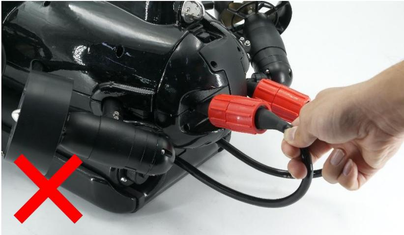
Do **NOT** pull the battery cable when recovery or carrying the submersible
