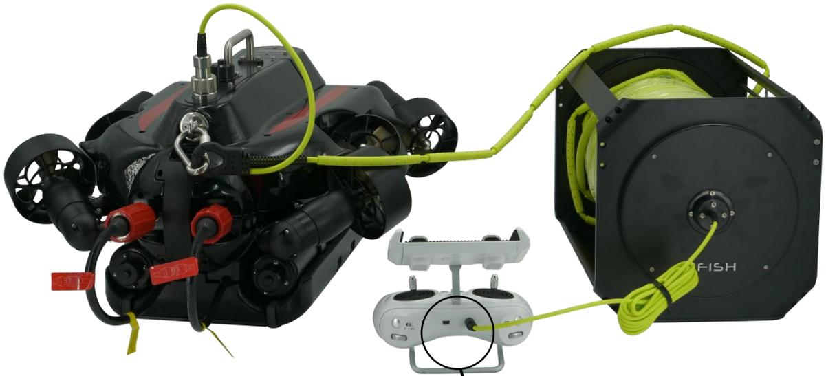
3.2.1. Plug the tether (3.5 mm head) into remote controller
