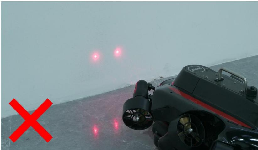
Do **NOT** turn ON the laser in air over 10 second, especially do **NOT** point the flammable materials
