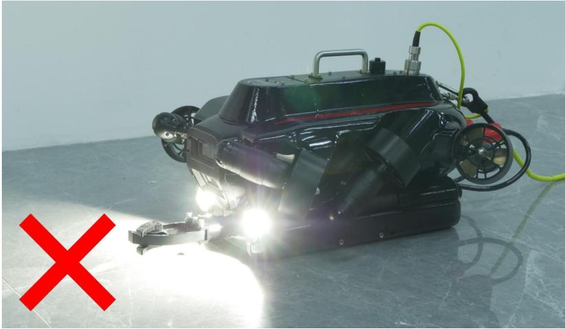
Do **NOT** turn ON the LED in air longer than 10 second to avoid over heating
