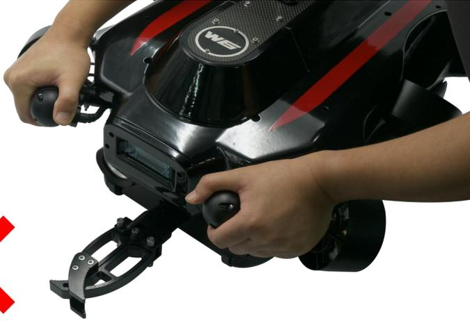
Do **NOT** holding the motor frame when carrying submersible
