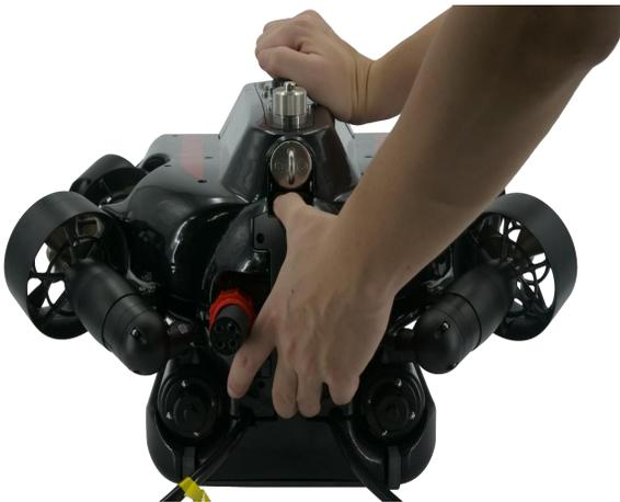
5.2.2. Press the battery release button and holding the back of submersible to unlock the battery, then pull out a little
